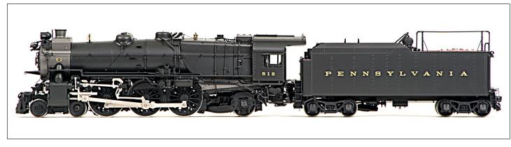
(above & cover) 'K-4sa' #612 with a special radio antenna equipped 130P75 tender. The most distinguishing feature of the 'sa' is the front-end throttle box mounted on the top of the smokebox. The 'sa' also had larger driving cylinders and a variety of other unique details, although the basic configuration is the same as the 'Post-War' version described on the previous pages. The K-4sa modified locomotives were the 'hot rods' of the class. (post 1952 service period)
