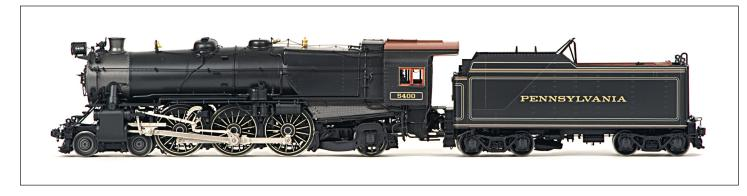
'As Built' 5400 series K-4 in full passenger dress, which includes striping on the cab, tender and wheel-sets. The tender is a 110P70 without stoker (1927-30 service period). The 'Early' version is the same as the 'As Built' configuration minus the striping. (1930-36 service period)
